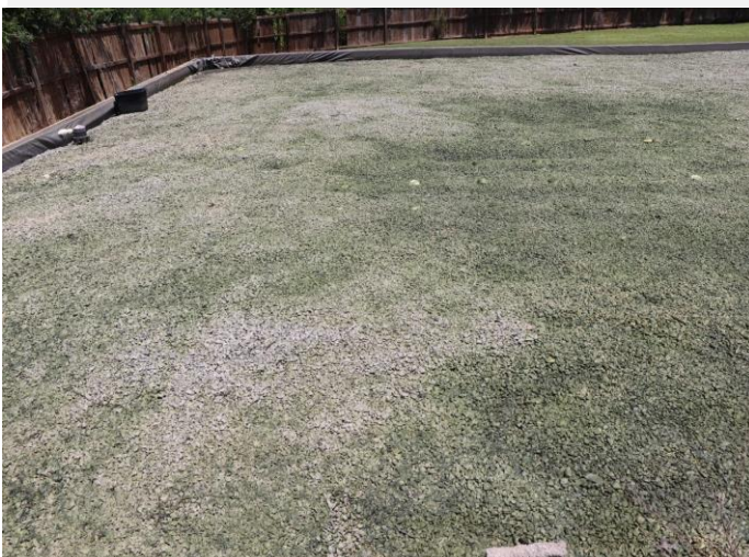
Before – Sand filter only treatment (impacted by algae)
