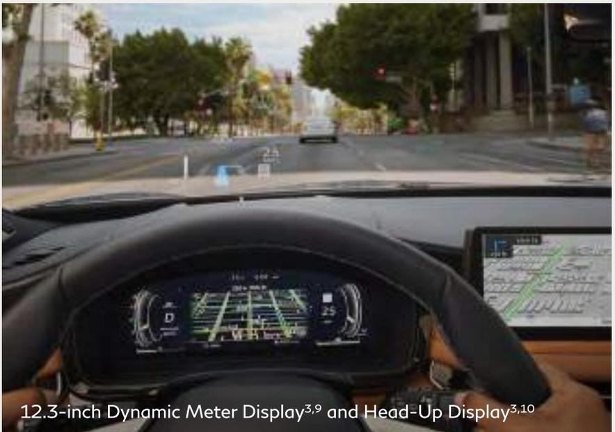
12.3-inch Dynamic Meter Display<sup>3,9</sup> and Head-Up Display<sup>3,10</sup>
