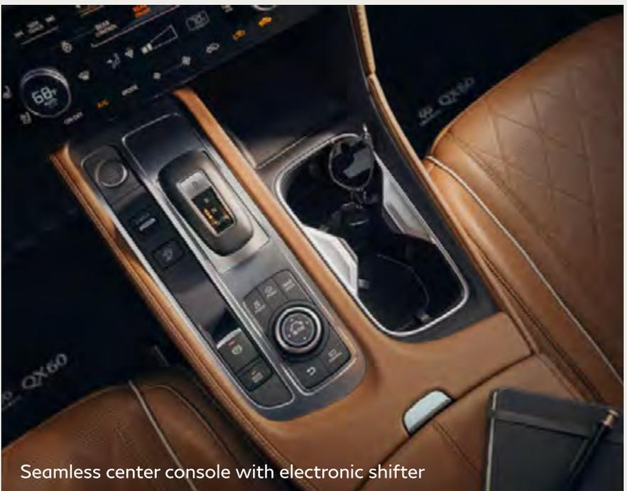
Seamless center console with electronic shifter
