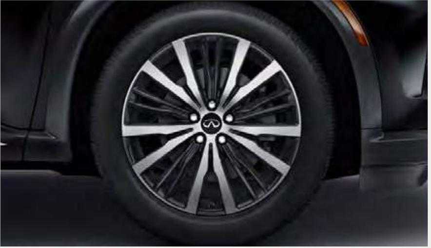
20-inch charcoal metallic machine-finished aluminum-alloy wheels
