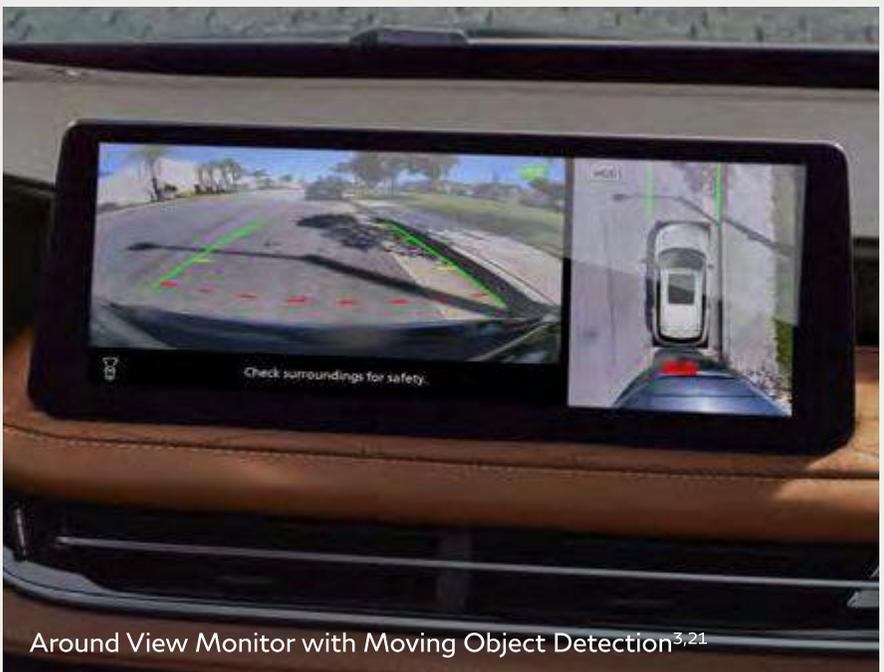
Around View Monitor with Moving Object Detection<sup>3,21</sup>
