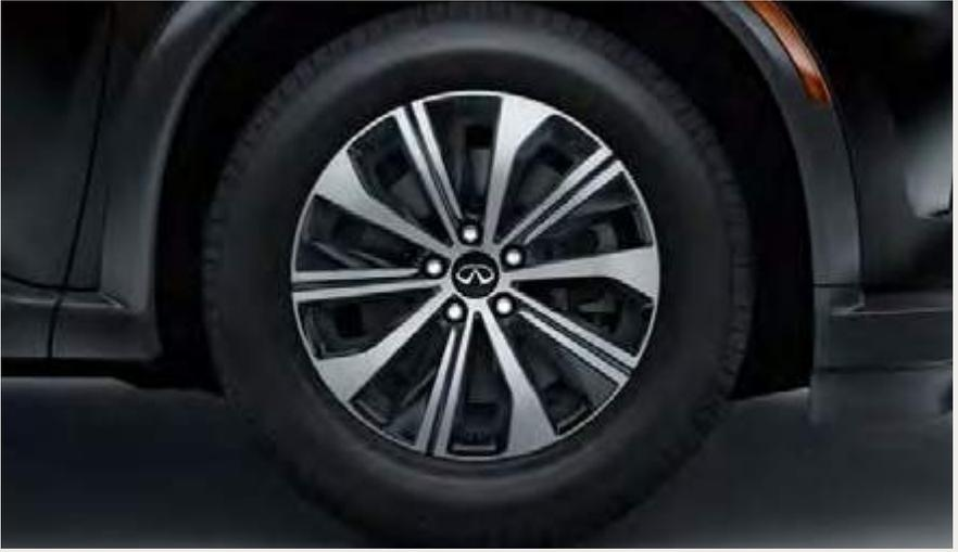
18-inch charcoal metallic machine-finished aluminum-alloy wheels (PURE)
