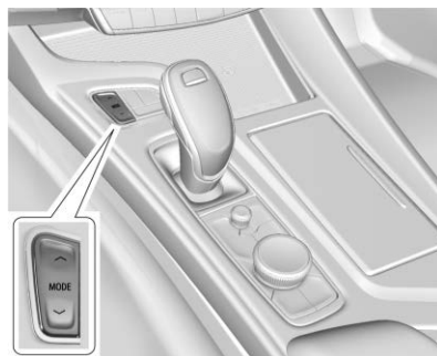
Driver Mode Control Switch
