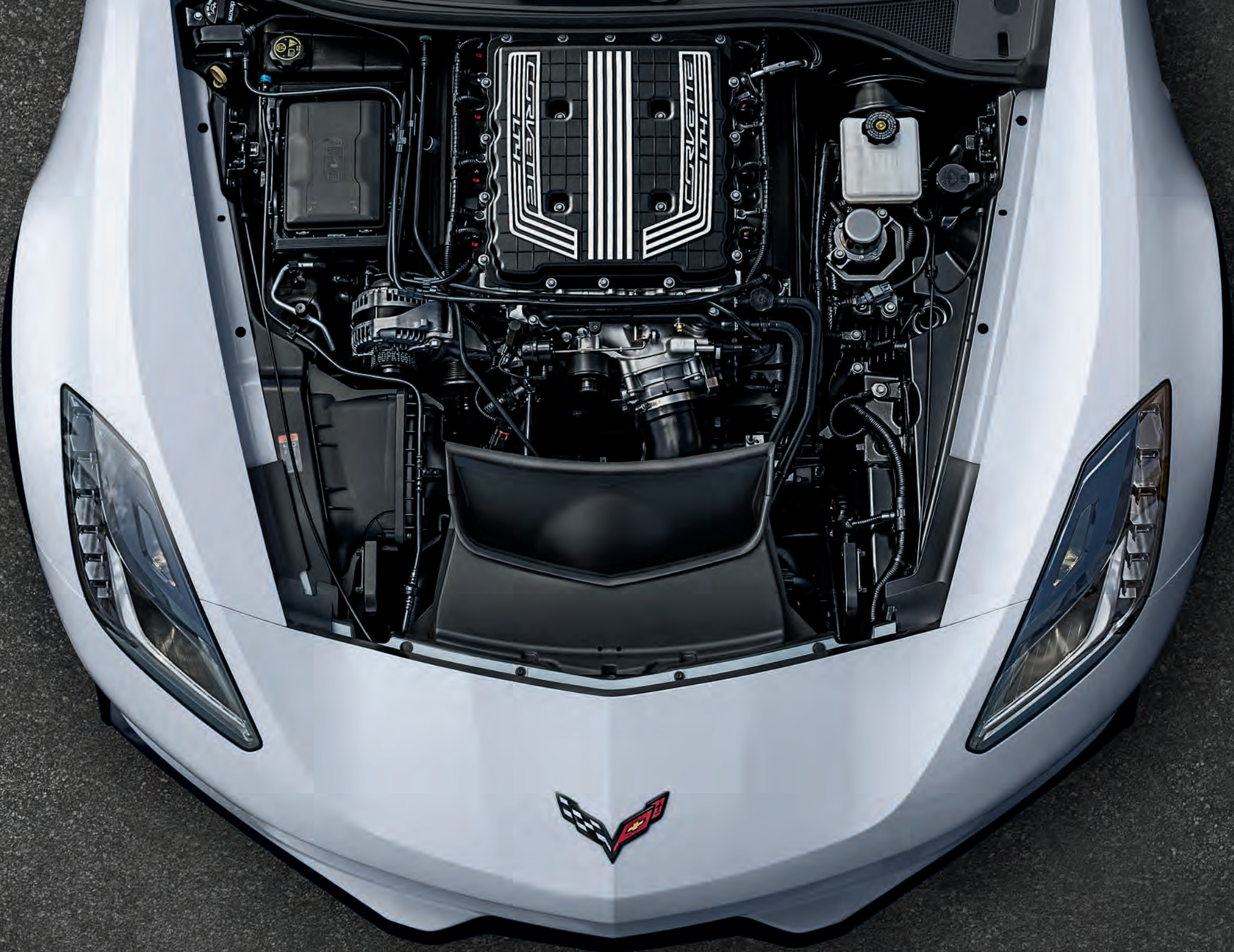
650-HORSEPOWER LT4 SUPERCHARGED V8 ENGINE. Standard on Z06.
